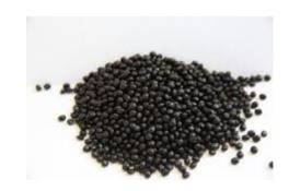
PLASBLAK PE2718 black masterbatch is not recommended for applications such as thin gauge or premium quality film extrusion.
