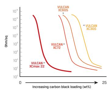
The graph demonstrates that the new VULCAN XCmax 22 specialty carbon black reaches the target conductivity at much lower loading levels.
