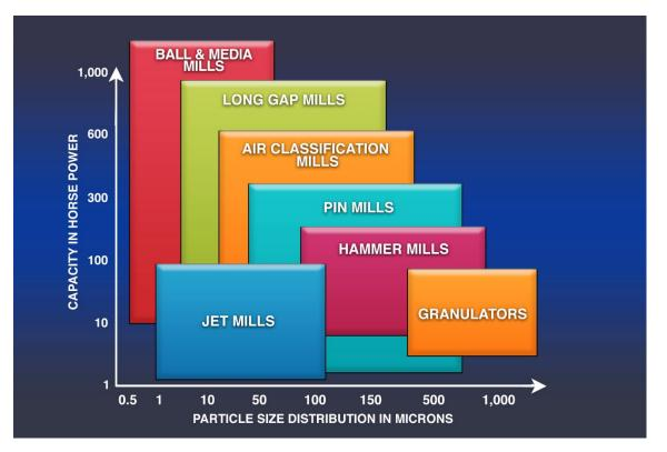
Figure 2: Particle size achievable by different types of mills designs. Source: <u>https://www.hmicronpowder.com/applications/size-</u> reduction/? vsrefdom=googleads&gclid=Cj0KCQiA95aRBhCsARIsAC2xvfwbZ3Dt48q6GXcONVkQThtQVkXYBU6ubsi5a7gba-<u>HZr33wlY3GIDUaAlSeEALw\_wcB</u>
