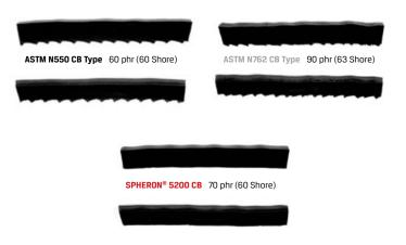
b) Good rubber properties with high resistivity (EPDM 100 phr, 0il 50 phr, S-cure system, Hardness ~60 Shore)
