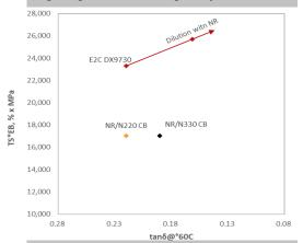
Figure 2. E2C DX9730 elastomer composite has high M300 and low hysteresis loss
