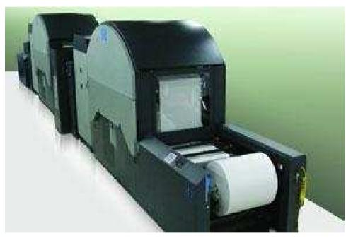
Speed: 122 m/min (2600 A4/min) Colorant: Aqueous pigments Printhead: TIJ, (HP) Resolution: 600 x 600 dpi Fixer: Yes
