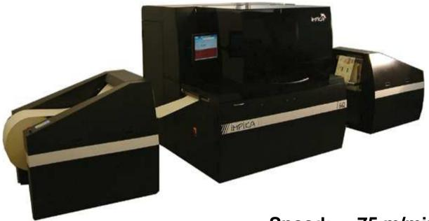
Target Markets: Direct Mail, Transactional, Labelling Speed: 75 m/min (1200 A4/min) Colorant: Aqueous dye or Pigment (4-6 colors) Printhead: Panasonic Resolution: 600 x 600 Fixer: none
