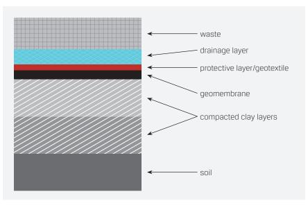
Fig 2. Cross-section of typical landfill multi-barrier concept
