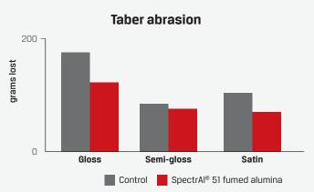
In Taber abrasion tests, the weight lost from the film when subjected to continuous abrasion is measured. The addition of fumed alumina to the model formulation can reduce the weight loss by up to 35%.
