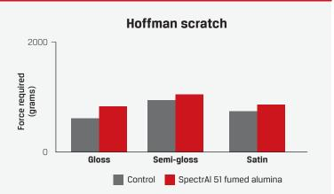
In Hoffman scratch tests, the amount of force required to cut the film down to the substrate is measured. The addition of fumed alumina to the formulation can increase scratch resistance in a range of finishes.
