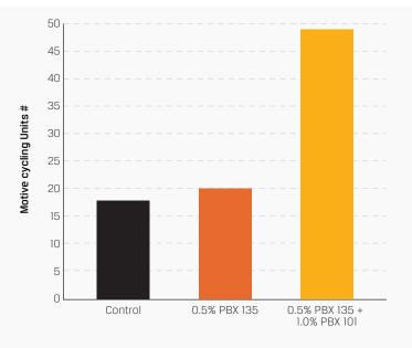
Figure 6: Deep discharge cycling of flooded batteries
