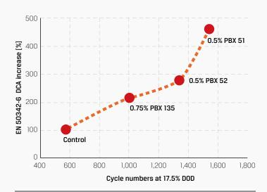
Figure 3: DCA and cycle life with our PBX performance additives vs. control electrode.
