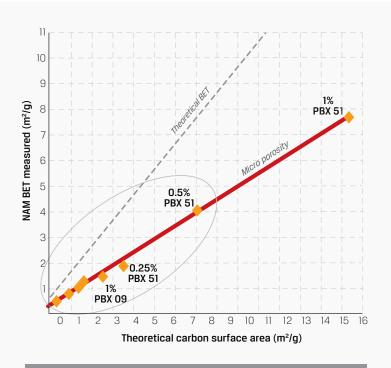
**Figure 8:** Effect of Cabot carbon additives on the negative electrode surface area
