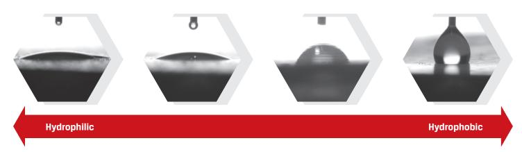
Figure 9: PBX carbon additives have surface properties ranging from hydrophillic to highly hydrophobic.
