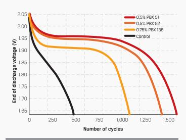
**Figure 4:** In continuous cycling tests at 17.5% depth of discharge, even at low loadings of 0.5-0.75%, PBX carbon additives significantly improve cycle life.
